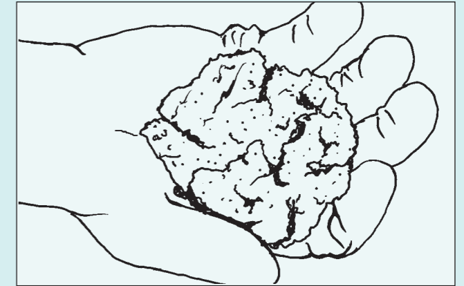
22. MIX AND DRY MORTAR
